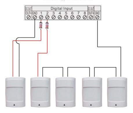
4) When digital input is NO and connected by end-of-line resistors, a 2.2K resistor needs to be connected in parallel.
