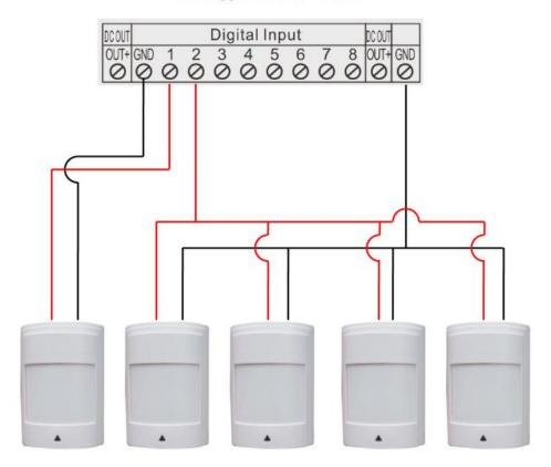
3) When the digital input is NC and the end-of-line resistors mode is selected, a 2.2K resistor needs to be connected in series.
