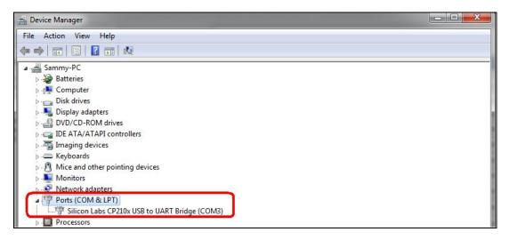
Step 3: Choose the correct COM port, then open configuration software
